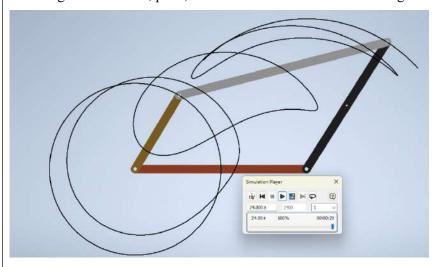
Design and Simulation of a Whitworth Quick Return Mechanism
